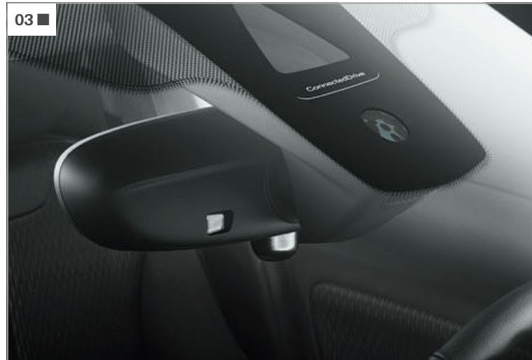
[ 03 ] The rain sensor including automatic headlight activation automatically switches on the windscreen wipers and the low-beam headlights.
