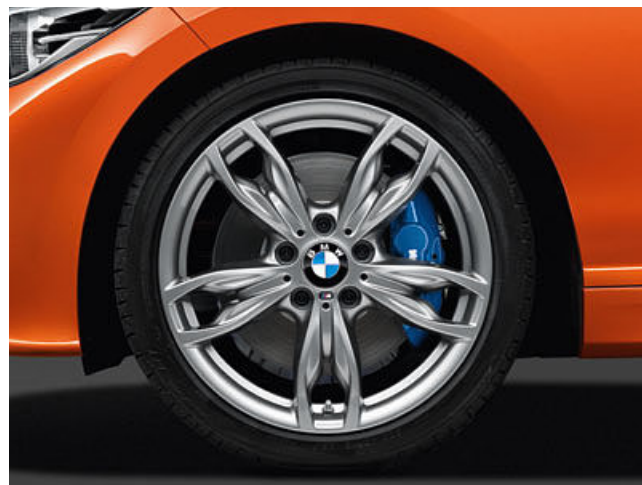
18" M light alloy wheels Double-spoke style 436 M with mixed tyres, front 7.5 J x 18 with 225/40 R 18 tyres, rear 8 J x 18 with 245/35 R 18 tyres.
